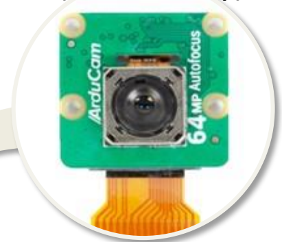
Camera Module 3 Raspberry Pi (ArduCam 64 mp)
