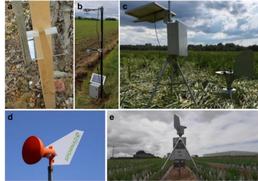
Fig. 1 Examples of spore samplers. a) Passive sampler comprising two microscope slides mounted horizontally on a wooden pole; b) rotating-arm impactors; c) Burkard 7-day recording volumetric sampler; d) funnel-like passive spore sampler from Spornado (courtesy of Kristine White and Yaima Arocha Rosete, Sporometrics); and e) Burkard high-volume cyclone (courtesy of Celine Hamon, Vegenov)
