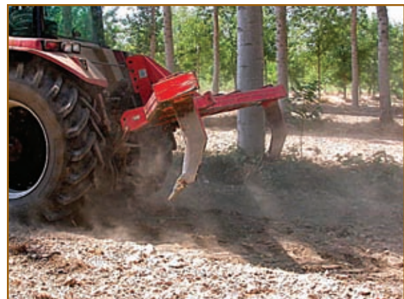
Photo 8: Research has shown that root-pruning (e.g. with the aid of a chisel plow) can limit underground competition between trees and crops.
